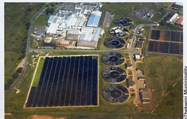
The Hammarsdale wastewater-treatment works has volumetric design capacity of 27 Ml/day.
